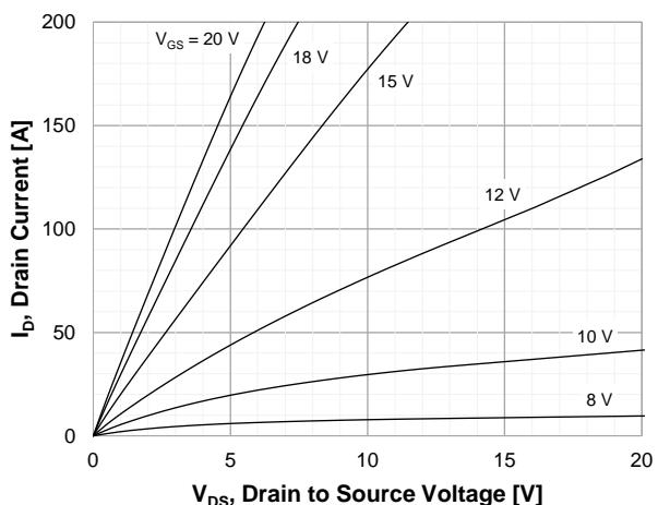
Figure 2. On-Region Characteristics  $T_J = 25^\circ\text{C}$
