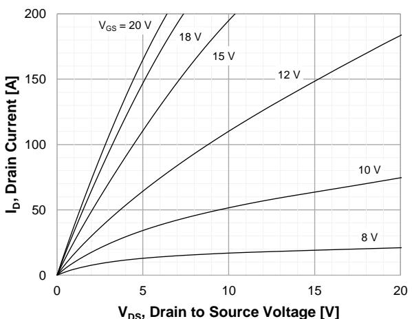
Figure 3. On-Region Characteristics  $T_J = 175^\circ\text{C}$
